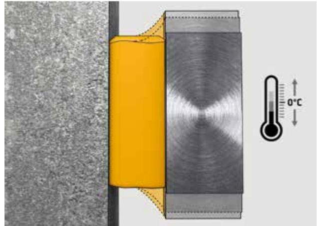
Compensating for different thermal expansion behavior of materials.
