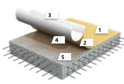
**The post-applied SikaProof® P-1201 system**, the membrane is installed into the freshly applied adhesive onto the prepared hardened concrete surface. There is no primer required, the full-surface and highly durable bond to concrete structure is created by the adhesive.
