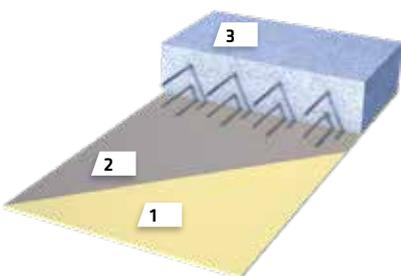
**The post-applied SikaProof® P-12 system** is installed by first peeling the release liner and sticking the membrane directly onto the hardened concrete surface. The full-surface bond to concrete is enhanced by the system primer, which ensures a durable adhesion to the concrete structure.
