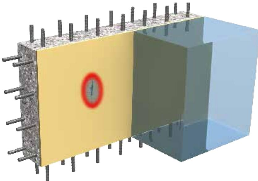
The "fully bonded technology" has been tested and approved in function tests according to ASTM and EN standards. Therefore the bonded membrane in combination with concrete is tested regarding the resistance to lateral water migration under a defined waterpressure over a specific periode.
