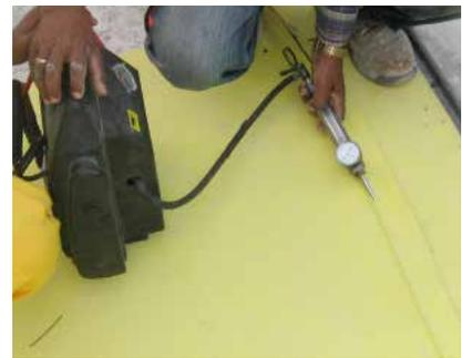
Air pressure testing using an air pressure pump, reverse flow valve and test needle that is inserted into a test channel between the seams of double seam welding (suitable for double seams only).
