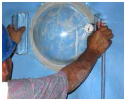
Vacuum testing using a vacuum bell and electrical vacuum pump for testing of details. After treating the seam edges with soap solution, the vacuum bell is firmly pressed over the area to be tested and the vacuum applied. Any leaks are clearly seen by bubbling of the soap solution under vacuum.
