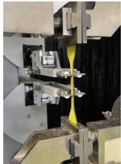
Behaviour after storage in hot water of 2 PVC membrane samples: stil conform with requirements according to ÖBV 4.7.
