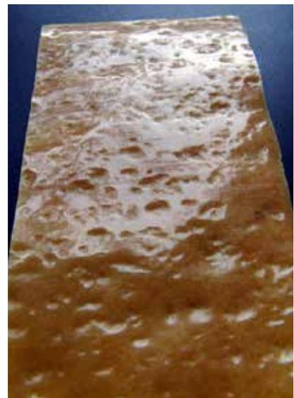
Comparison of lab testing (simulation) with 41 years old real exposed samples (validation), taken from the Reussport tunnel in Switzerland.
