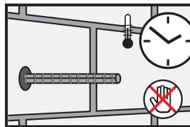
During the resin hardening time the anchor must not be moved or loaded. Wash tools immediately with Sika® Colma Cleaner. Wash hands and skin thoroughly with warm soap water.
