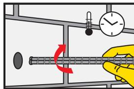
Insert the anchor with a rotary motion into the filled drill hole. Some adhesive must come out of the hole.
