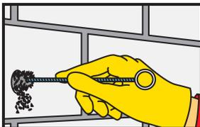
The drill hole must be thoroughly cleaned with the special steel brush (brush at least 2x). The diameter of the brush must be larger than the diameter of the drill hole.
